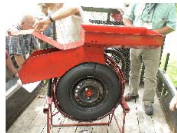
where the walnuts drop in and closest at the exit tray. The hulls drop out the bottom. This home made huller was on display at Bud Luers walnut orchard at the 2010 NNGA annual meeting, Wooster, OH.
