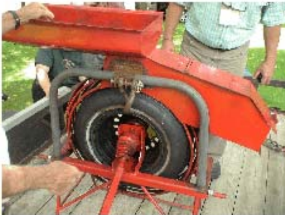
Three point hitch walnut huller made using a small auto front wheel drive axil and powered with the tractor PTO. Walnuts are fed in the top try. Wheel in top picture turns CCW, bottom pix CW. Hulled walnuts come out the lower try, hulls drop out the bottom. The 5 rebar are spaced furthest from the tire
